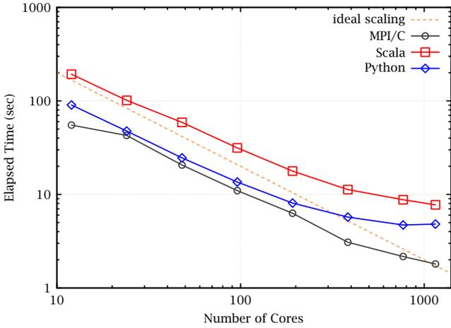
Fig. 2. Strong scaling results for COOLEY (log scale).
