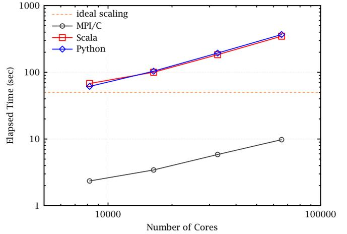
Fig. 3. Weak scaling results for THETA (log scale).
